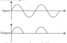
Output frequency of a half wave = input frequency = 50 Hz
